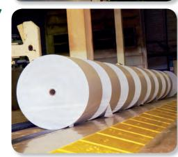
In 2017, Volga JSC mastered the production of reduced-weight newsprint - 40 g/m2. The advantage of lightweight paper is the increased paper area per roll.
